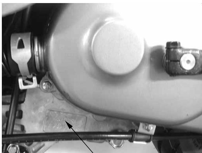
Location of Engine Serial Number
